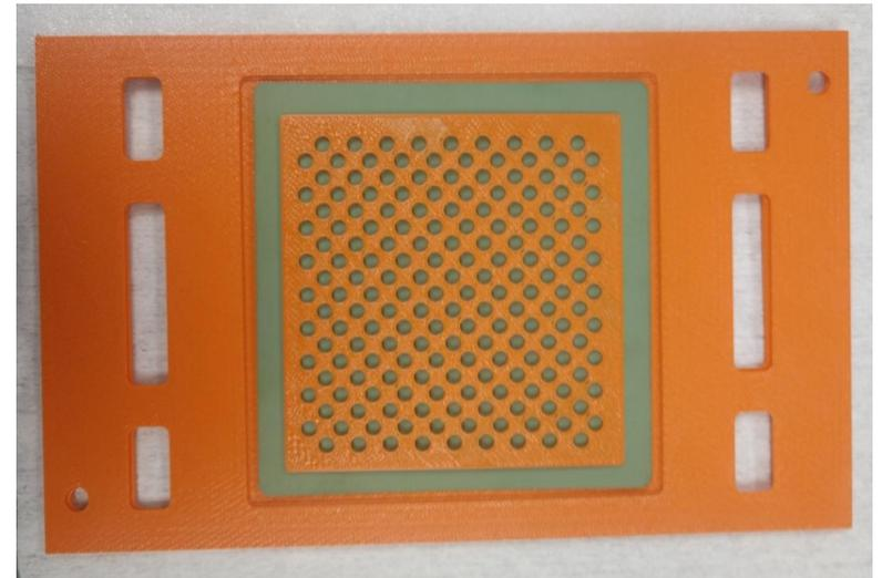
A 3D printed interconnect overlaid with a cell
