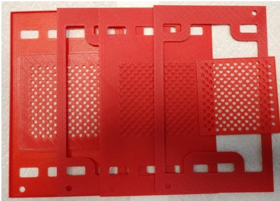
A set of 3D printed interconnect layers
