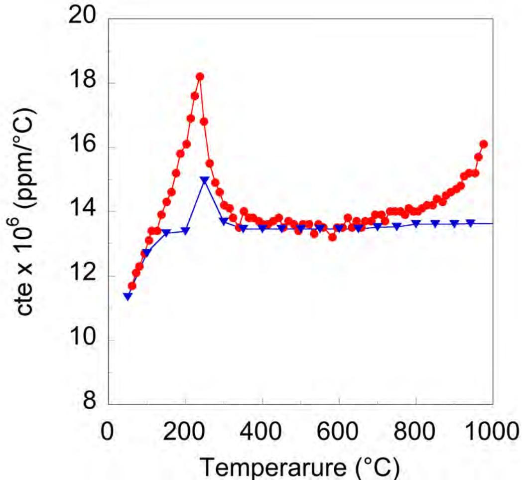
Coefficient of thermal expansion of NiO. **Blue triangles** from: CINDAS LLC, Purdue Technology Center- Aerospace, 1801 Newman Road, Suite 104B, West Lafayette, IN 47906-4510. **Red circles** from: Mori M, Yamamoto T, Itoh H, Inaba H, and Tagawa H. "Thermal Expansion of Nickel-Zirconia Anodes in Solid Oxide Fuel Cells during Fabrication and Operation," *J. Electrochem. Soc.*, **Vol. 145**, No.4, April 1998 pp.1374-1381.
