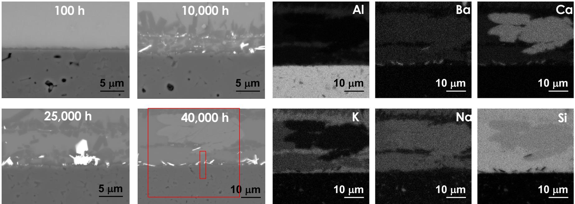
Structure and chemical changes at interfaces region by using SEM – three new phases formed at the SCN-Al<sub>2</sub>O<sub>3</sub> interface. Ba-Ca-O based (bulk in center), Ba-Si-O based (bright lath), and K-Al-Si-O based (dark lath); GB diffusion in substrate was apparent.
