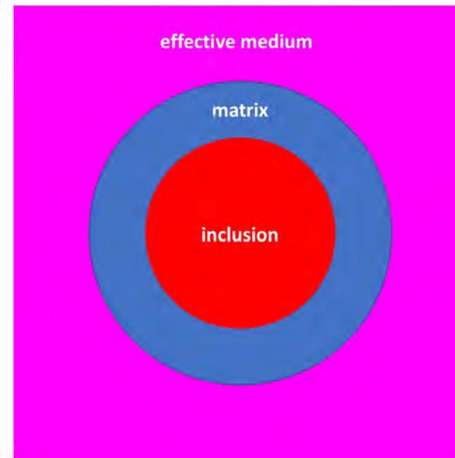
A micromechanics model has been developed to calculate the effective properties of a 3-phase composite (NiO, YSZ and porosity) as a function of temperature.
