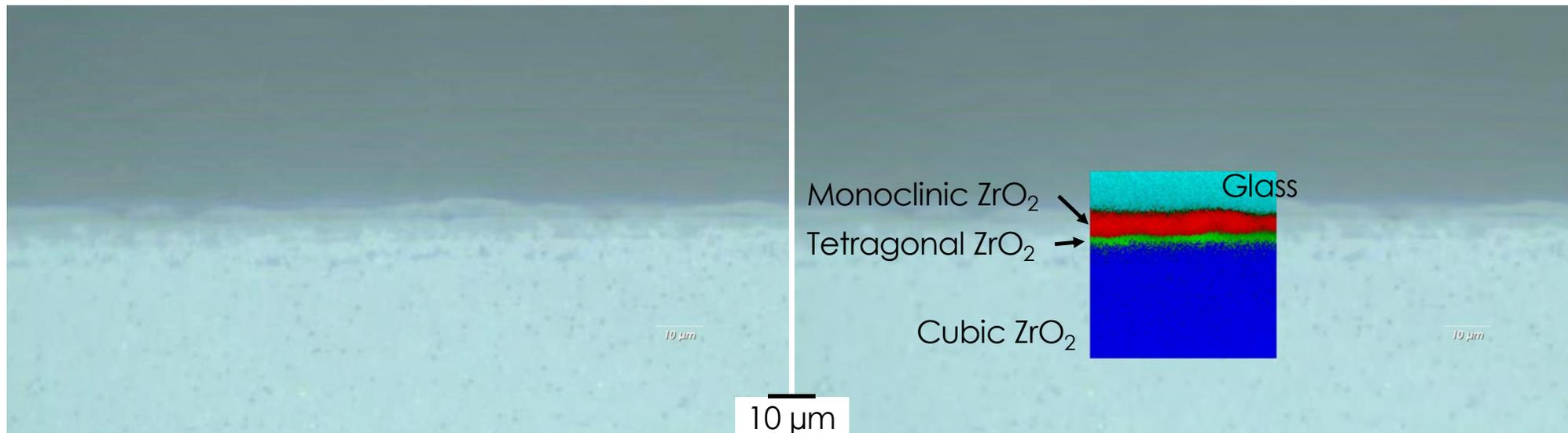
The diffusion of yttria into the glass, results in a transformation of the substrate from cubic to tetragonal to monoclinic ZrO<sub>2</sub>.
