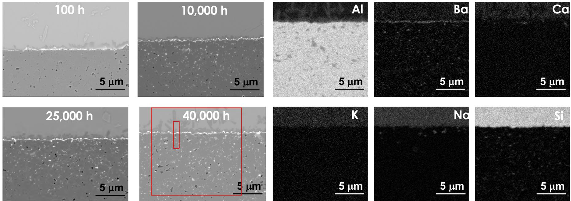
Structure and chemical changes at interfaces region by using SEM – two new phases formed at the G6-Al<sub>2</sub>O<sub>3</sub> interface: Al-Na-Si-O based (dark lath at interface) and Ba-Al-Si-O based (thin bright layer). Significant GB diffusion was noted.
