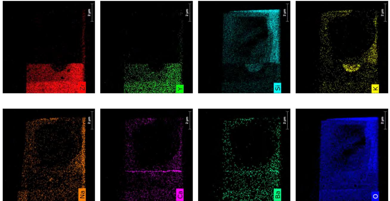
Substrate: Zr-Y-O with a half sphere void with Si-K
