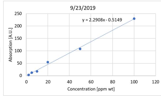
Calibration curve for UV-vis measurements on standard chromate concentrations
