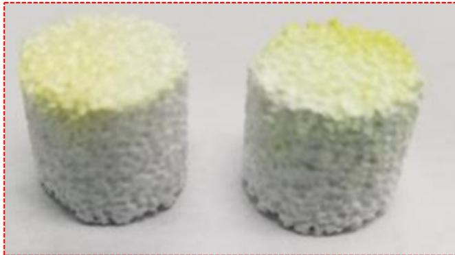
Filter after 500 h test with flowing humidified air over stainless steel (left) and  $\text{Cr}_2\text{O}_3$  (right) at  $750^\circ\text{C}$ .
