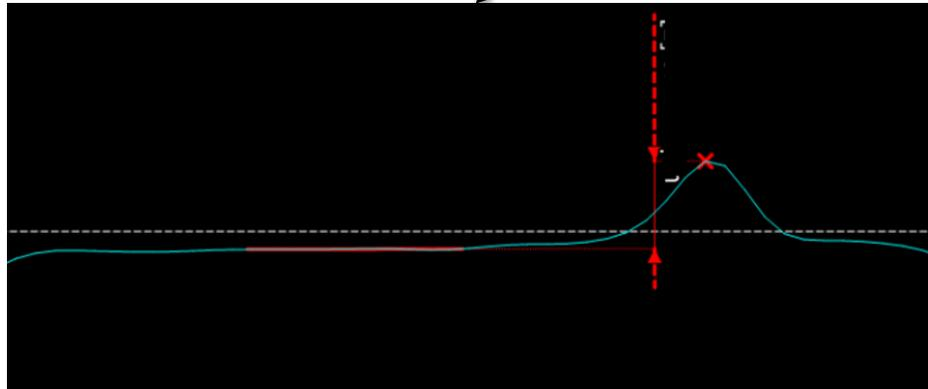
D) Cross section height profile that can be quantitatively analyzed, correlated to performance, and used during manufacturing QC
