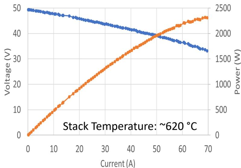
— Stack Voltage (V) — Stack Power (W)
