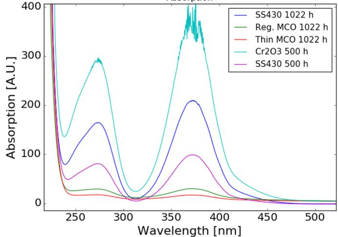
UV-vis measurements for chromia, uncoated sample and multiple types of MCO coated samples
