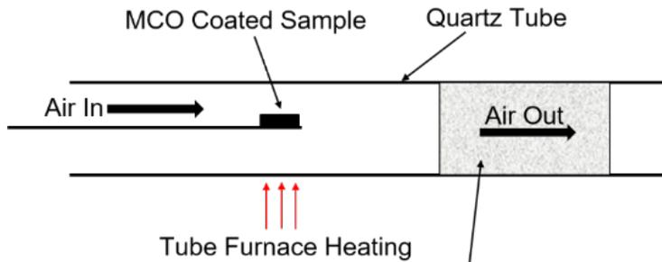
Gaseous Cr species released from the samples were captured using Na-carbonate coated alumina filters placed downstream from the samples\*
