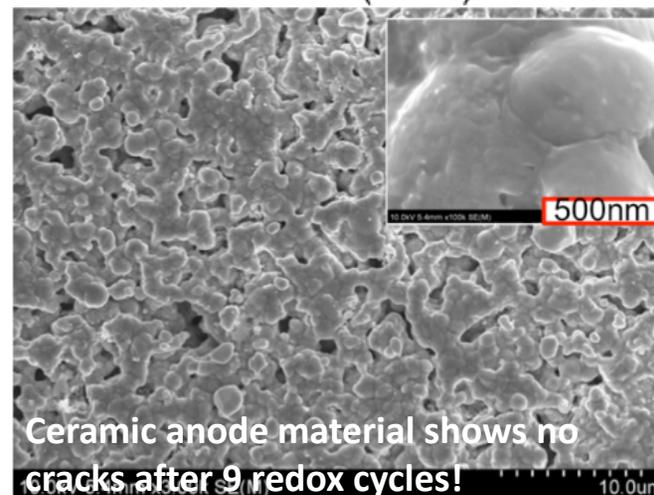
**Ceramic anode material shows no cracks after 9 redox cycles!**
