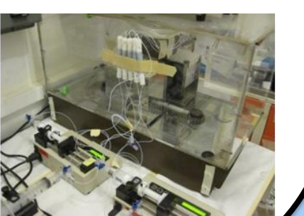
Uranium extraction with Osorb-TBP media -94% recovery from 1000 ppm U -Successful strip/cycle
