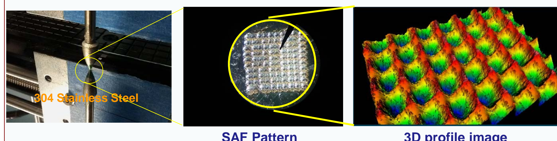
Schematic of Selective Area Forging and machine setup
