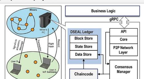
POC's DSEAL secure decentralized messaging and transaction platform allows detecting and mitigating false command, false sensor data, and other cyber threats for the achievement of a robust, reliable energy system
