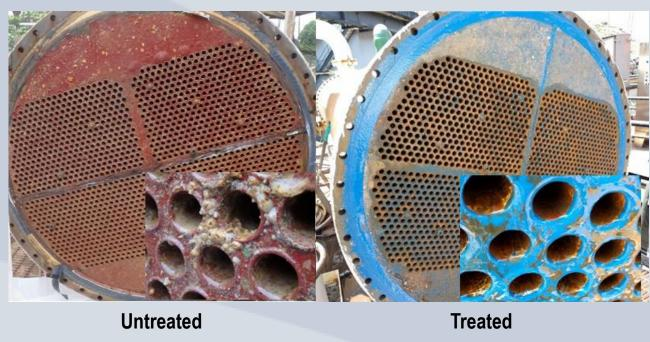
Heat transfer efficiency was greatly improved after HeatX<sup>™</sup> application. Seawater outfall temperatures were reduced by nearly 100%, allowing for generator turbines to be run at maximum rated load for extended periods of time, when they were typically capped at 50% due to insufficient cooling to keep up with thermal load requirements.
