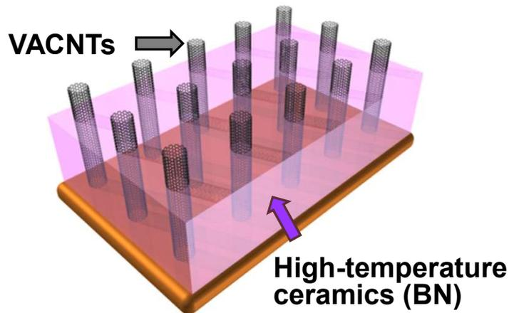
**VACNTs:** Electrical and thermal conductive channels.
