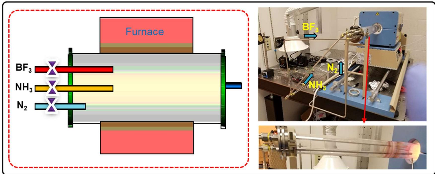
$\text{BF}_3$  and  $\text{NH}_3$  are separately fed into the hot zone to prevent undesired reaction at low temperature
