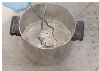
Parts dipped in liquid nitrogen
