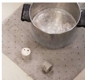
Parts dipped in liquid nitrogen
