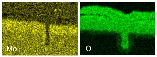
Oxide scale at specimen surface
