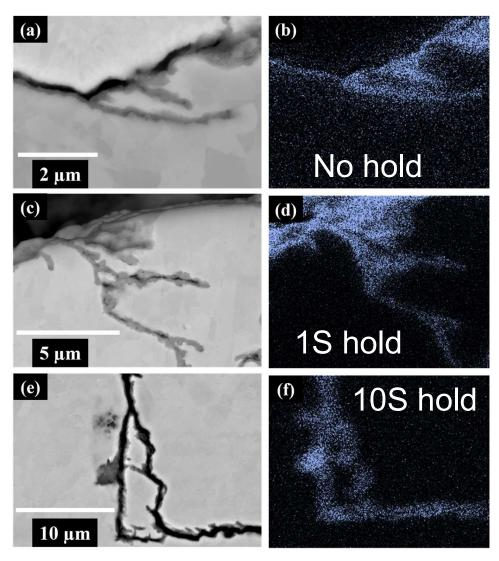
Depending on the scale (Fe or Cr-rich), oxidation at 550°C can be very fast Oxidation-induced crack closure?
