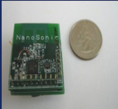
NanoSonic's Wireless Sensor Modular Hardware, "M" Shape Antenna Operates at 2.4 GHz band with 25 Possible Channels
