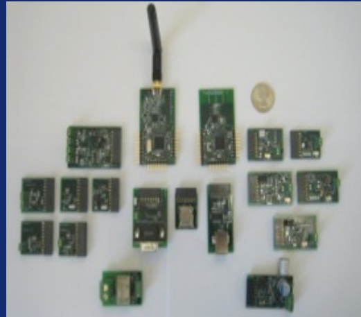
NanoSonic's Wireless Sensor Modular Hardware, "M" Shape Antenna Operates at 2.4 GHz band with 25 Possible Channels
