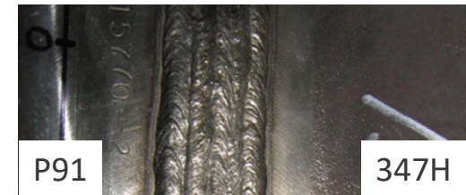
At Edison Welding Institute (EWI) By Gas Tungsten Arc Welding (GTAW). With Post Weld Heat Treatment.
