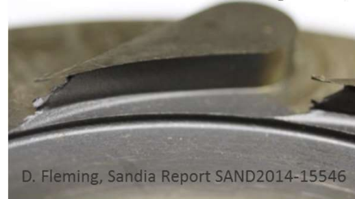
Erosion of turbine nozzle in sCO 2 test loop
