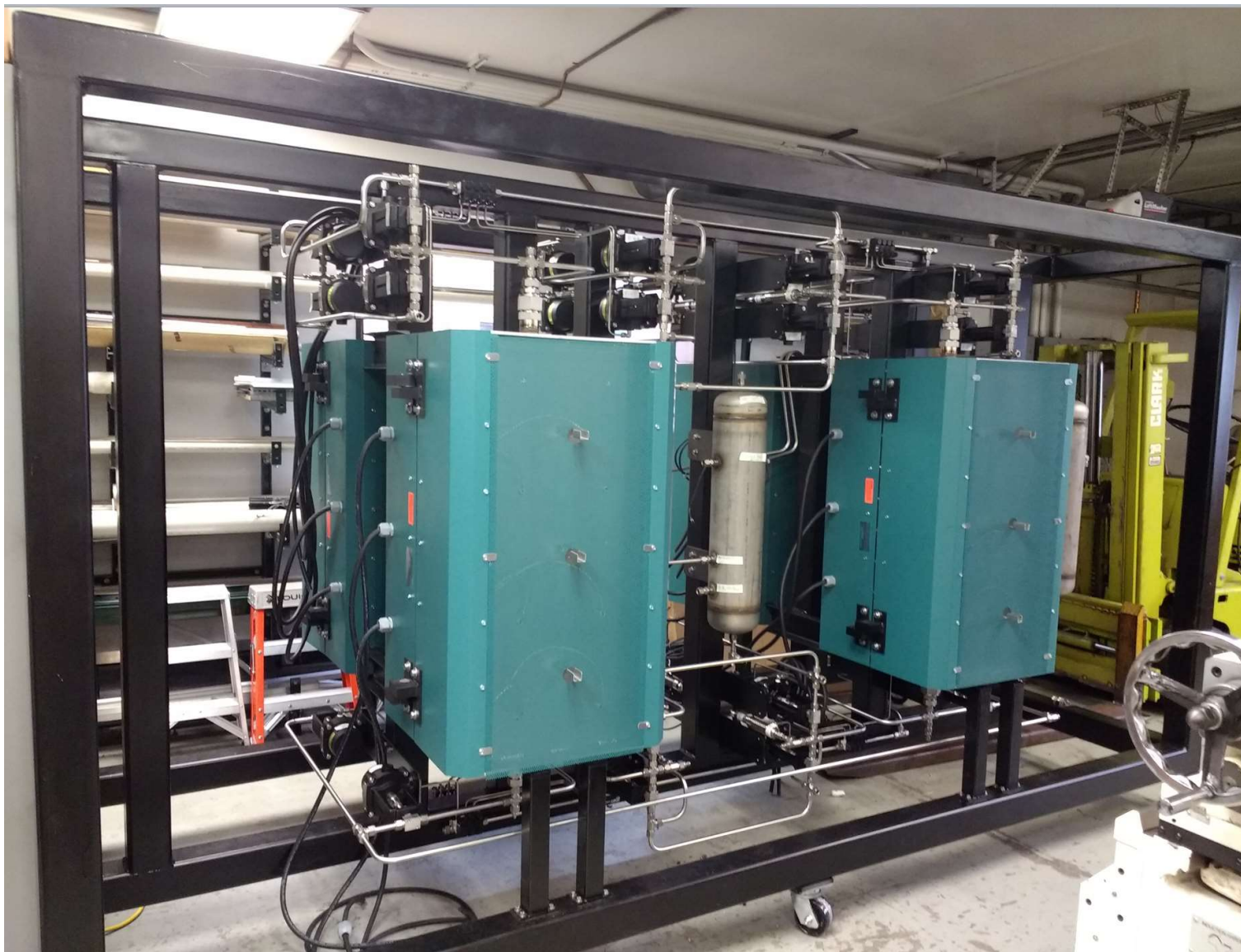
1 kg/hr O 2 Generation System
