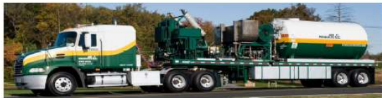
Express Services Pumper Truck Estimated Usage : LIN, 20-85 GPM (110,000 to 475,000 SCF/Hr), Pressure < 150 psig
