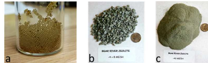
Figure 1. Solid sorbents evaluated in batch equilibrium studies. a) Dowex® G-26 resin (Dowex), b) granulated clinoptilolite (G-Clino), c) powdered clinoptilolite (P-Clino)
