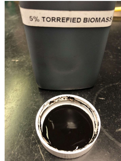
Coal/Water Slurry with 5% torrefied biomass
