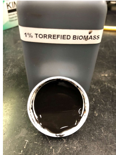
Coal/Water Slurry with 1% torrefied biomass
