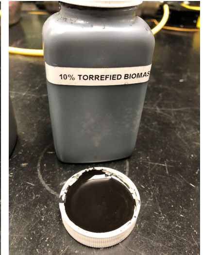
Coal/Water Slurry with 10% torrefied biomass
