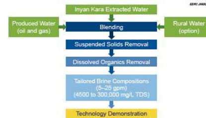
Conceptual extracted water treatment flow diagram.
