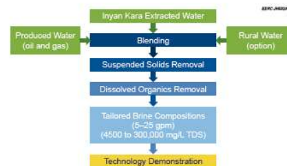
Conceptual extracted water treatment flow diagram.
