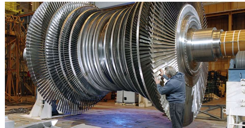
Figure: Turbine blade inspection
