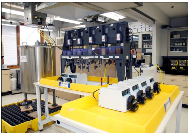
Solvent extraction upgrading of coal ash pregnant leach solution.
