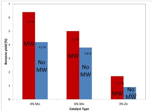
**Methane to benzene reaction (700 C):** Benzene yield increased significantly in the presence of microwave; Catalyst: 4% Mo, 6% Mo, and 3% Zn supported on HZSM5
