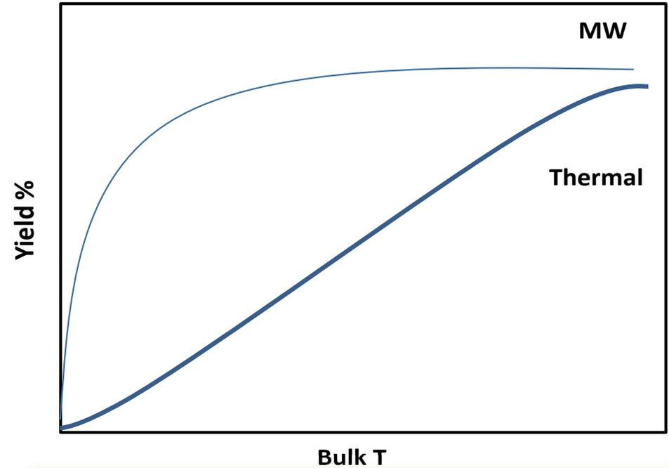
MWs allows for *selective heating* of reacting species/sites, which can lower bulk T...can result in higher product yields for rxns that favor lower equilibrium temperatures
