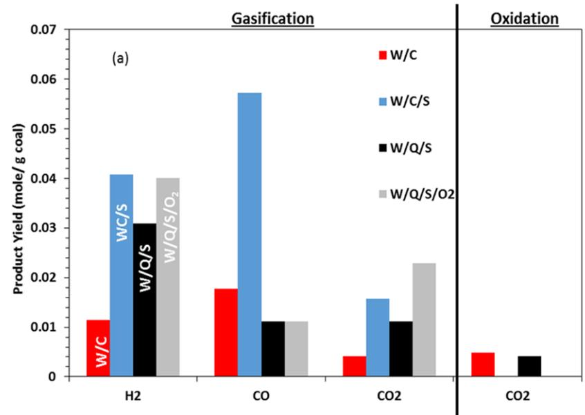
Wyodak coal(W) gasification with calcium ferrite (C) and steam (S) and comparative gasification data with quartz (Q) and 0.75 vol.% gaseous oxygen (O<sub>2</sub>)
