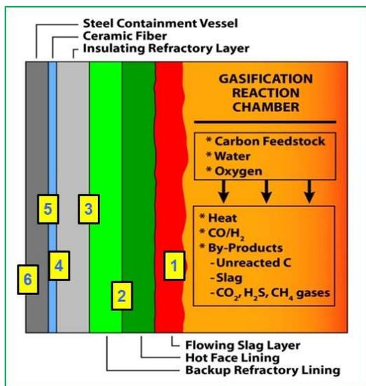
**Air cooled slagging gasifier = Refractory temperatures for a given carbon feedstock flow rate and HF brick thickness (9 or 0 in).**
