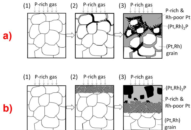
Surface attack of Pt/Rh thermocouple wire caused by phosphorus. Two types of diffusion occur, **a)** P and Rh through grain boundaries, and **b)** P and Rh through grain lattice, depending on the wire composition. Efforts are directed at preventing attack such as this.
