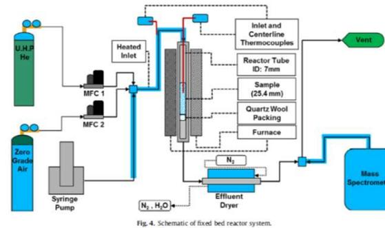
Fig. 4. Schematic of fixed bed reactor system.
