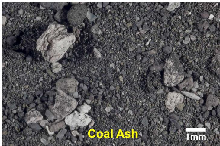
Ash agglomeration/fouling has impacted every gasification process. It is influenced by: 1) the gasification process, 2) the carbon feedstock, 3) process temperature, and 4) process flow rates.
