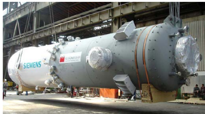
A Siemens SFG™-500 Gasifier is shown (left) with matching Feeder Vessel (below).
