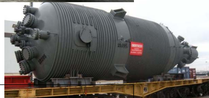
A Siemens SFG™-500 Gasifier is shown (left) with matching Feeder Vessel (below).
