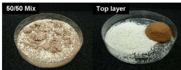
Figure 4. Results of tests with CK46 meta-kaolin – 50/50 mix of meta-kaolin with deposit (left), meta-kaolin as a top layer over deposit (right)
