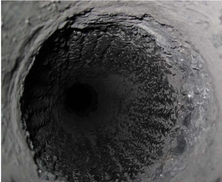
Slag layer retained after 38 hours on low ash petcoke (view looking down from gasifier injector)
