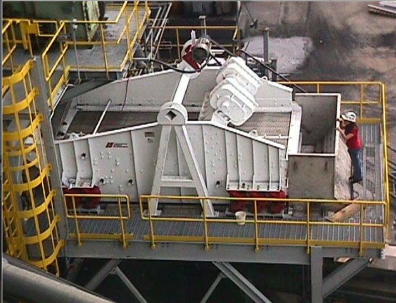
Moving forward, we are installing a new larger coarse slag screen during the current outage. It will receive our slag directly from our lockhopper and drag flight conveyor, eliminating double handling. The screen will separate the coarse, low carbon, marketable material from the fuel and fines portion. The plant is already configured to recycle this fuel and fines to slurry preparation and the coarse material can be sold with little or no post-treatment.
