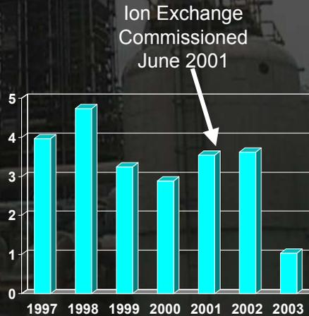
Last year, we reported commissioning our ion exchange system to remove heat stable salts from our MDEA solution. We were experiencing some accelerated corrosion in areas of the amine system that are typically vulnerable.
