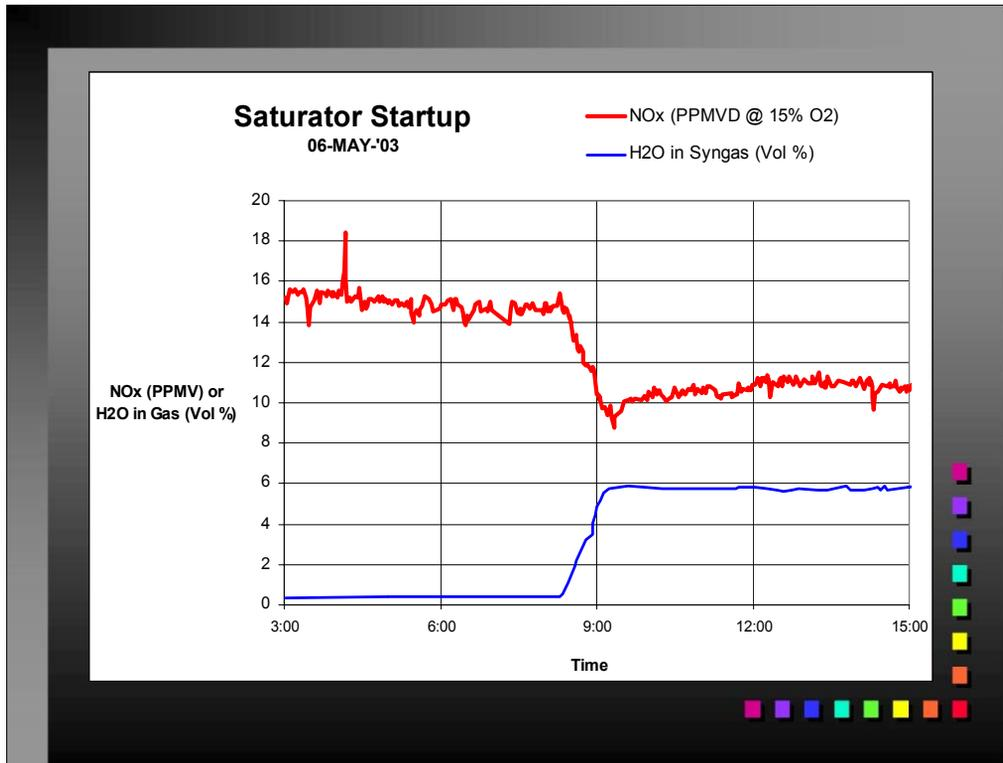
Polk was required to reduce NOx emissions from 25 to 15 ppmvd (15% O<sub>2</sub>) by July, 2003. As we discussed in last year's paper, we elected to do this by supplementing diluent nitrogen with syngas saturation using low level waste heat. The system was successfully commissioned in early May. This shows the initial run. The saturator has been operating trouble-free ever since, enabling us to comply with the new permit limit.
