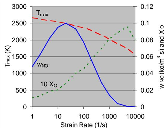
Figure 3.2.2: Strain rate effects, adapted from Sanders et. al. [15].  $w_{\text{NO}}$  = NO formation rate,  $X_{\text{O}}$  = O-atom mole fraction,  $T_{\max}$  = peak temperature
