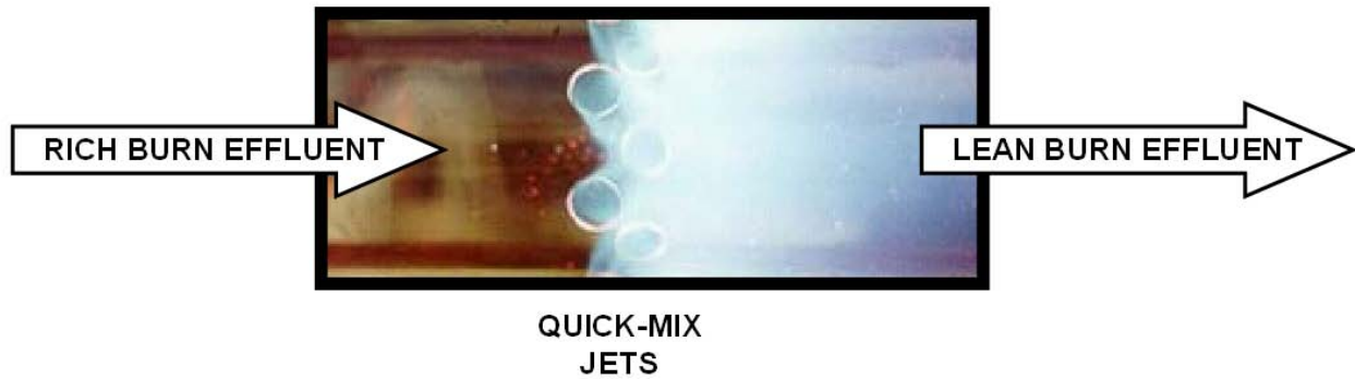
Fig. 5. Laboratory Model Combustor
