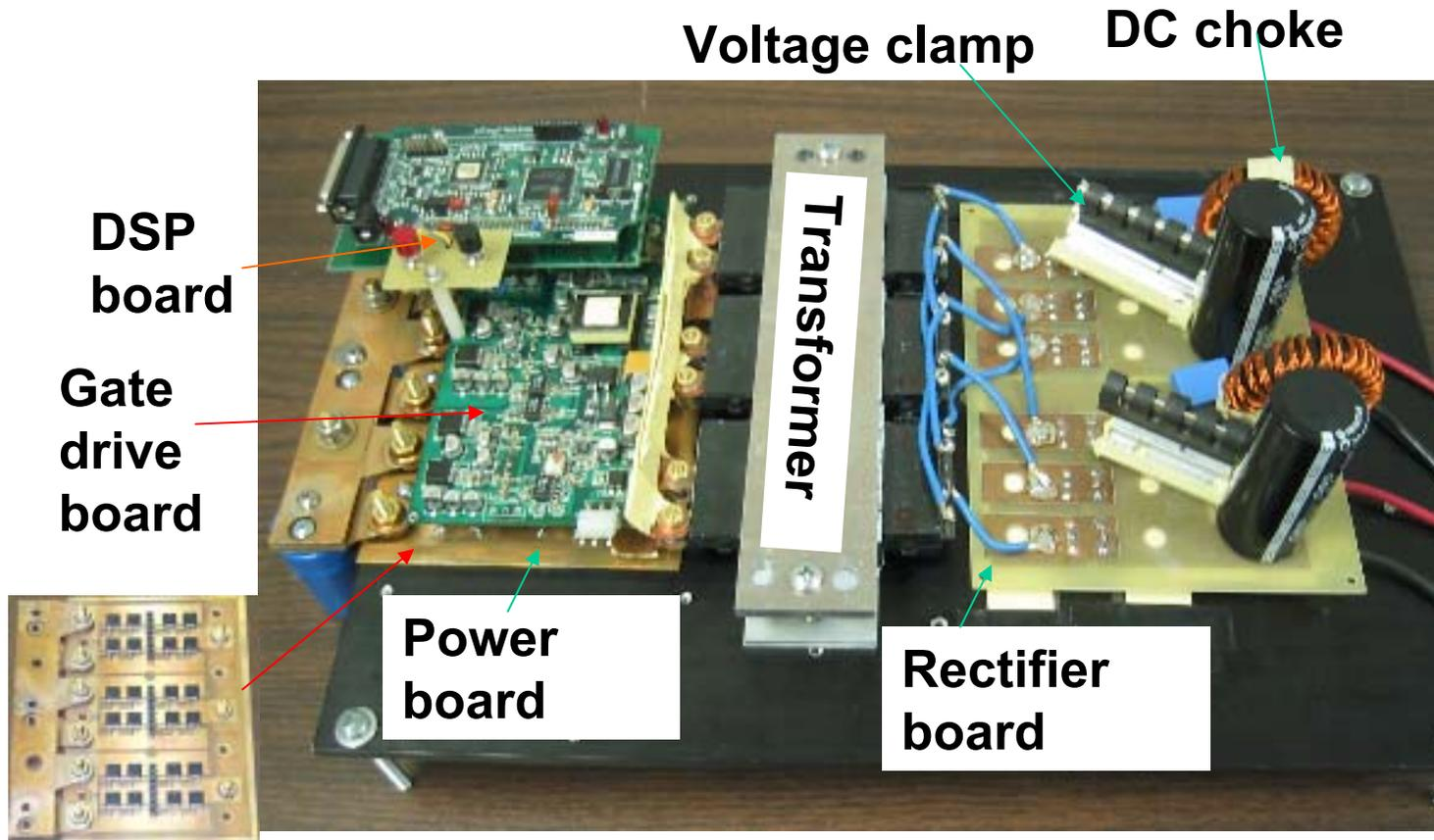
**Note: The power switch has four TO-263 devices in parallel**
