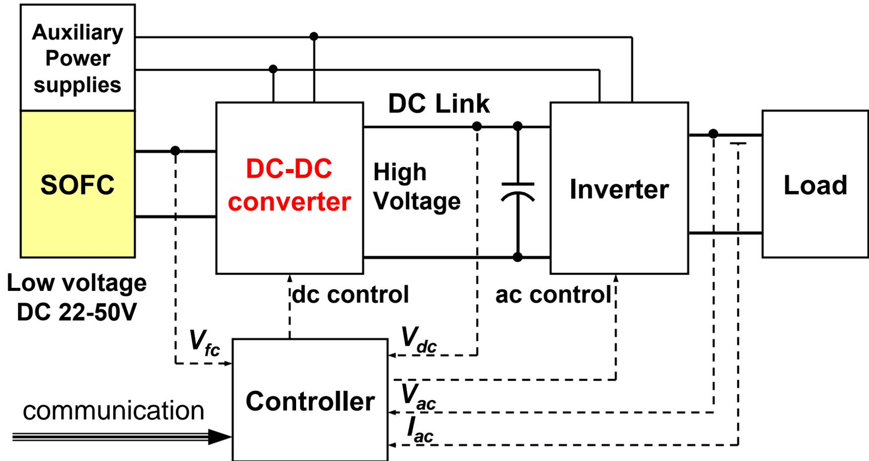
**The DC/DC converter is the most crucial electrical interface to the fuel cell source**
