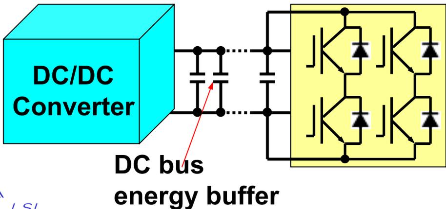
Adding energy storage capacitors at the DC bus not only smoothes out the inverter load transient, but also reduces fuel cell current ripple proportionally.
