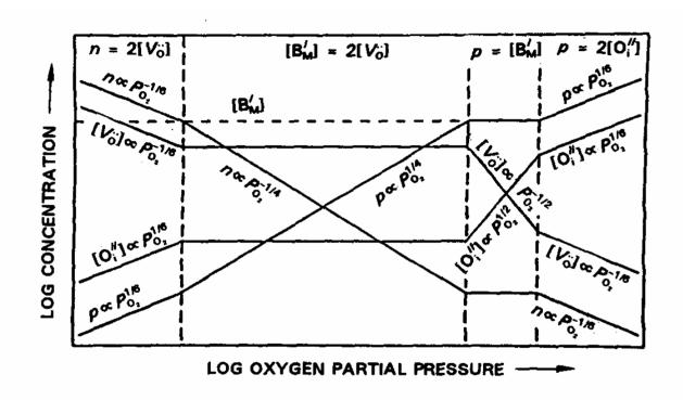
Figure 3.3. Variation of defect concentration as a function of oxygen partial pressure for a  $MO_2$ - $B_2O_3$  system [3.17]
