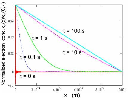
Before the zirconia electrolyte is introduced to a  $P_{O_2}$  gradient (i.e., at t = 0), the concentration distribution is flat. After the  $P_{O_2}$  gradient is introduced, a new concentration distribution gradually established.
