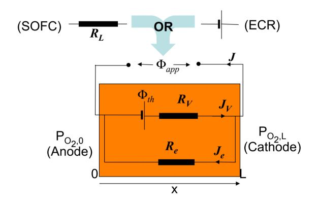
$$J = (\bar{t}_{ion} \Phi_{th} - \Phi_{app}) \overline{\sigma}_{tot} L^{-1} = \eta \overline{\sigma}_{tot} L^{-1}$$
