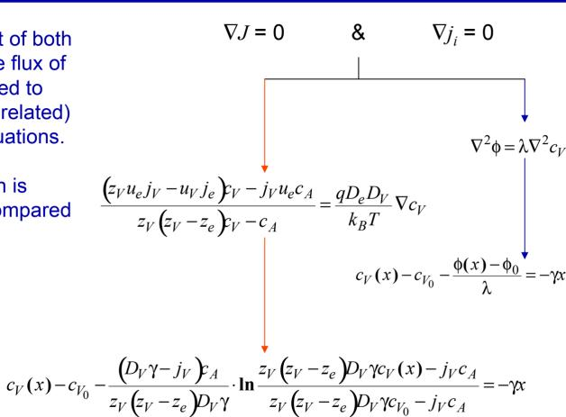
$$\gamma = \frac{\phi_L - \phi_0}{\lambda L} - \frac{c_{V_L} - c_{V_0}}{L} \qquad \lambda = \frac{\left(z_V - z_e\right)k_B T}{z_e q c_A}$$
