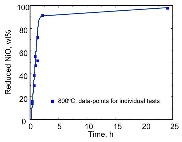
Reduction of NiO measured for different samples. Samples were reduced for a different period of time at 800°C in 4%H2-96%Ar gas mixture
