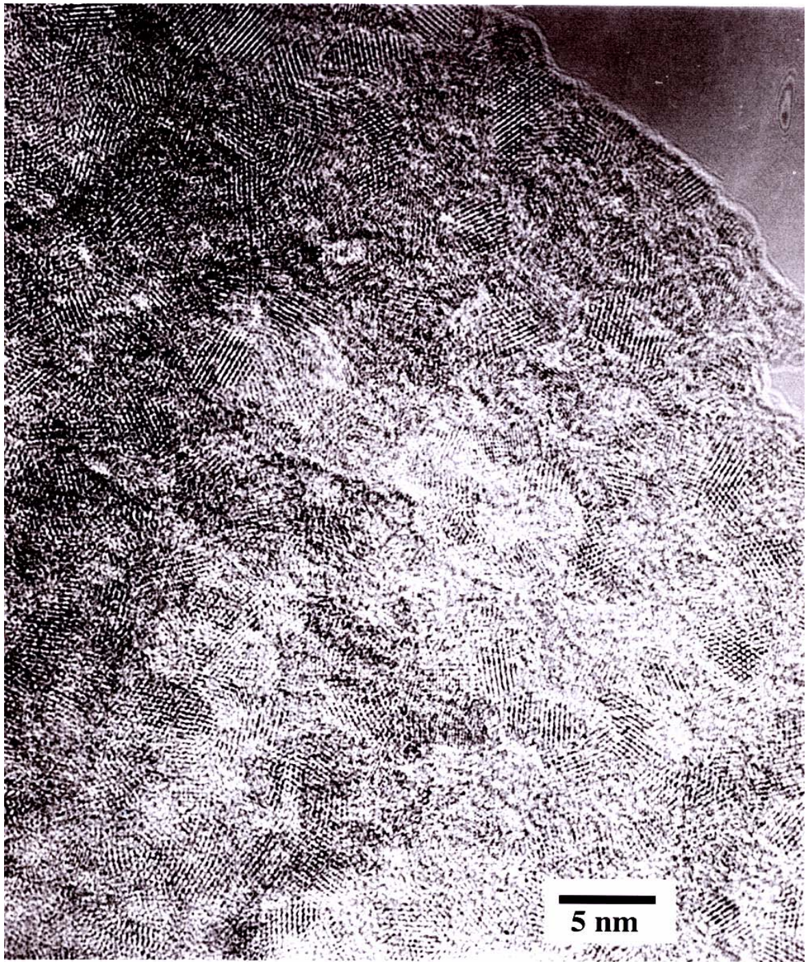
YSZ thin film annealed at 400°C for 2 hrs. d_g = 6\text{nm}
