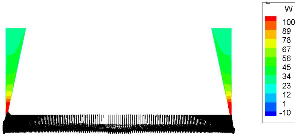
Axial Velocity Distribution at Combustor Inlet
