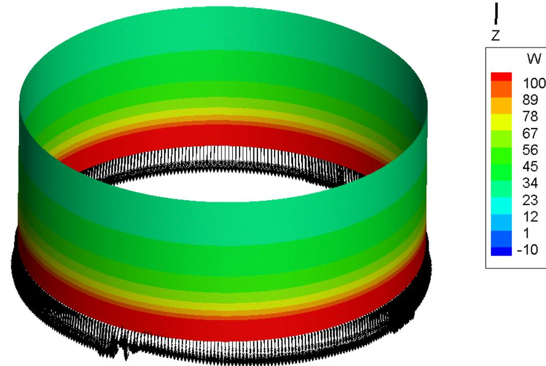
Axial Velocity Distribution at  $R = \text{const}$
