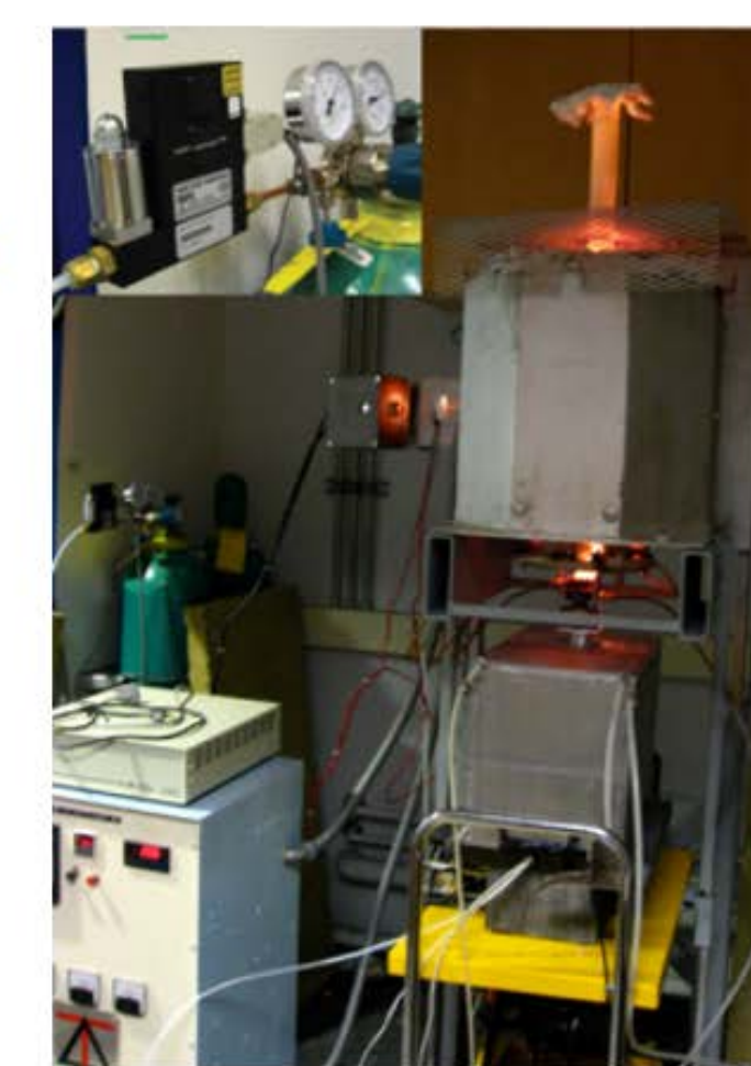
(a). Illustration of the high velocity testing apparatus that will be built to characterize volatilization under high velocity steam 2 .
