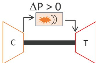
“Constant Volume” Combustion incorporates a Pressure Gain with combustion
