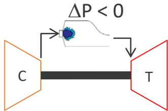
Conventional “Constant Pressure” Combustion has pressure loss across combustor
