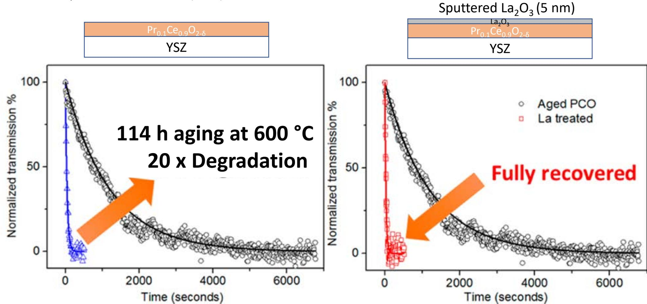
La layer traps Si → surface exchange rate recovered
