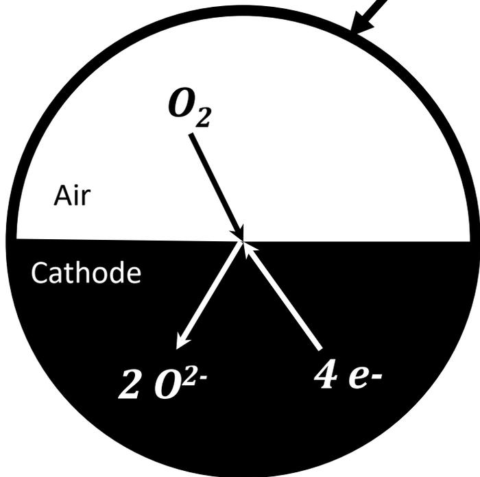
Oxygen Reduction Reaction limited by solid/gas surface exchange reaction rate
