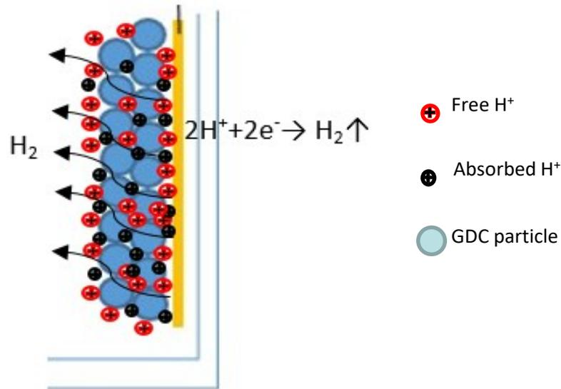
Fig.4 Schematic of reaction near cathode
