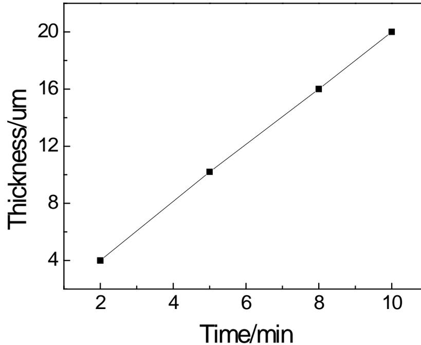
Thickness as a function of time for a GDC/ethanol suspension, under constant-voltage conditions (100V) when using polypyrrole coated YSZ as the cathodic electrode
