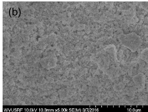
Cross-section and (b) surface morphology of GDC layer before sintering
