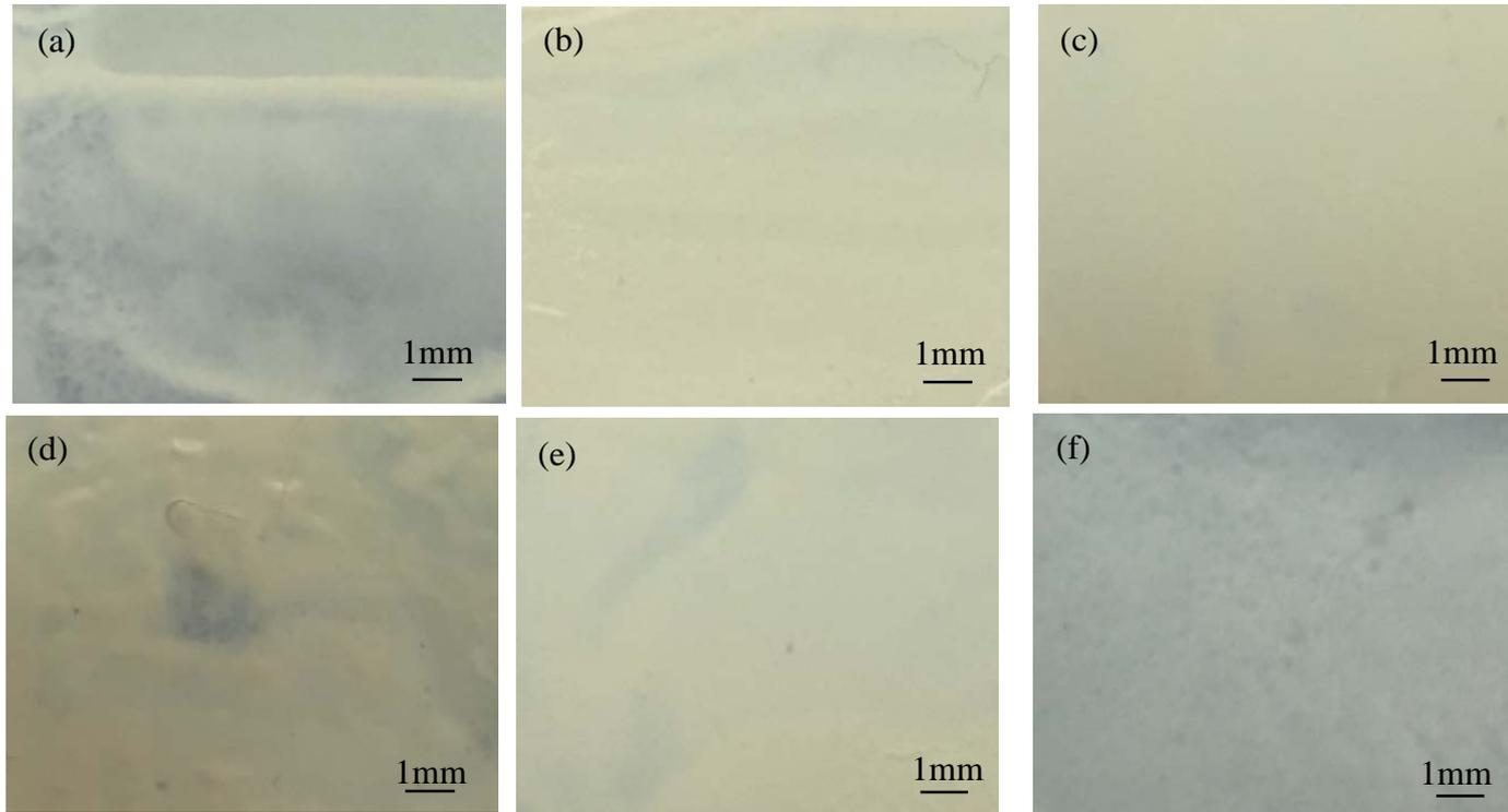
The deposit for 10 mins as a function of applied voltage (a) 60V, (b) 80V, (c) 100V, (d) 120V, (e) 140V and (f) 160V
