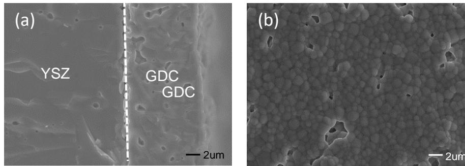
Fig.12 (a)cross-section and (b) surface morphology of GDC layer with 2mol%  $\text{FeO}_{1.5}$  after sintering at 1300°C
