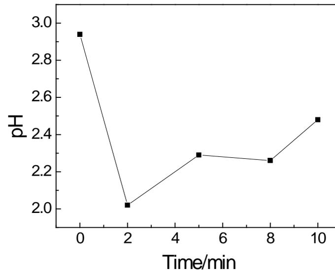
(a) current and (b) pH near the cathode as a function of time under constant voltage
