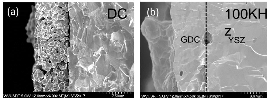
Fig.13 cross-section of GDC layer with 2mol%  $\text{FeO}_{1.5}$  formed by (a)DC and (b) 100kHz AC EPD after sintering at 1250°C
