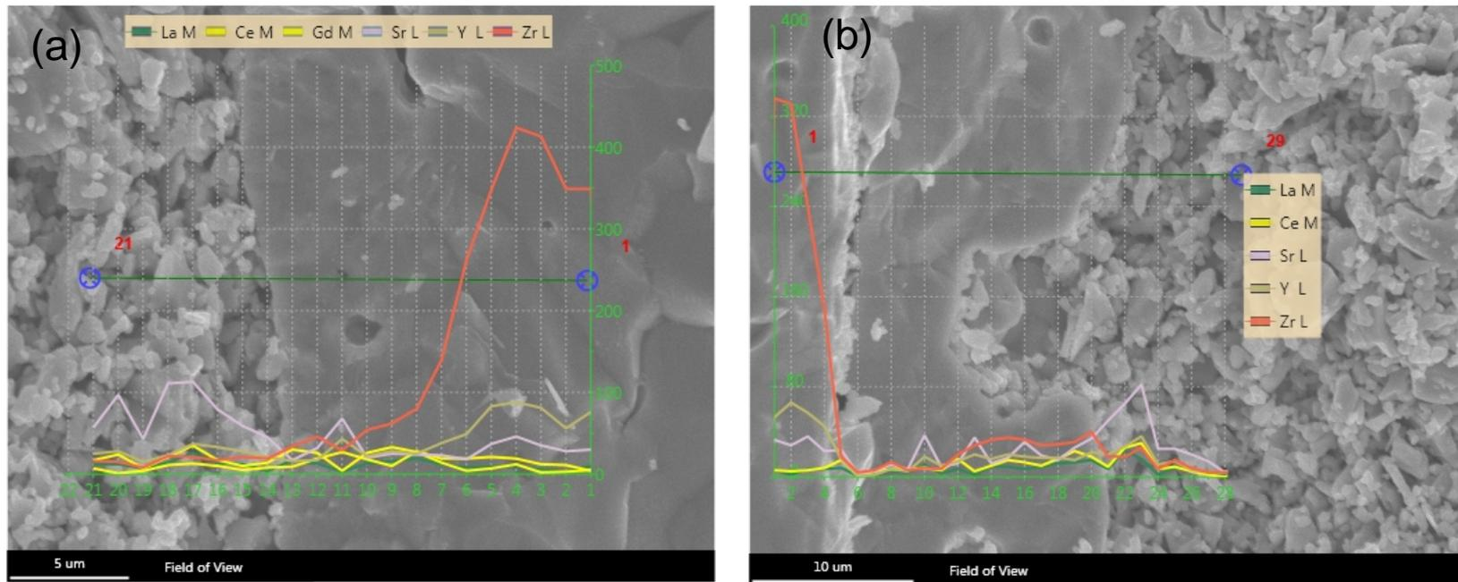
Fig.17 EDAX analysis of LSCF/GDC/YSZ before after long-time stability test
