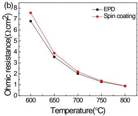
EIS at 750°C and (b) temperature dependence of Ohmic resistance of symmetric cell with GDC layer with sintering aid formed by spin coating and EPD
