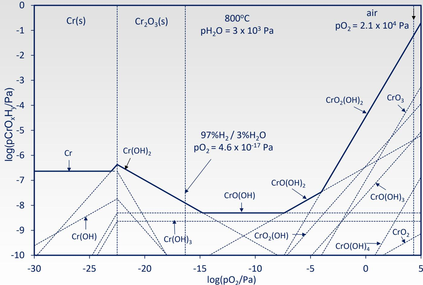
Vapor pressures higher in oxidizing conditions
