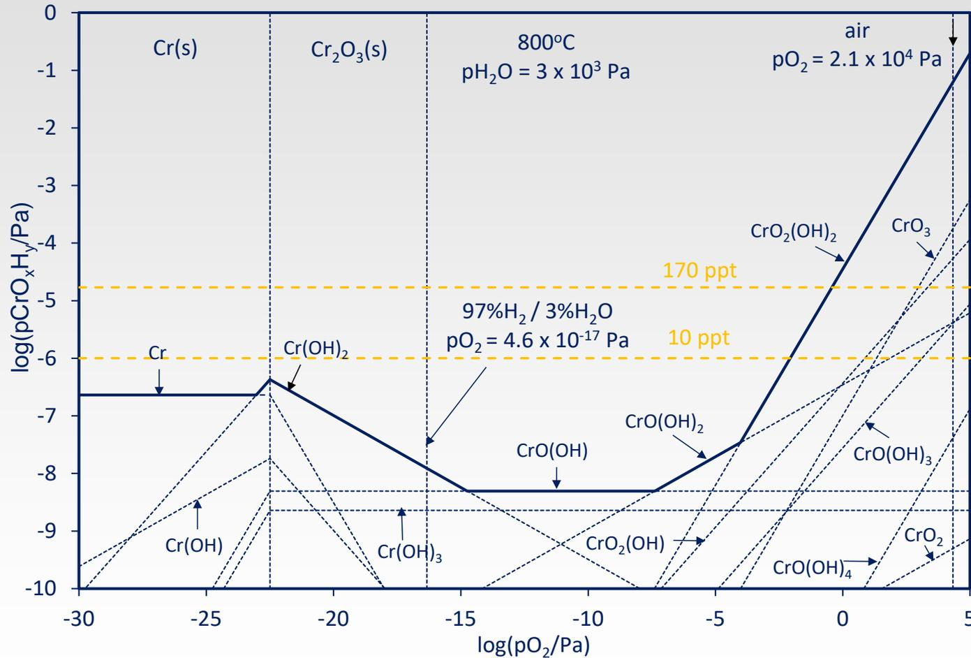
Vapor pressures higher in oxidizing conditions
