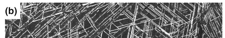
Nimonic 263 samples were aged at temperatures of 750°C, 800°C, 850°C, and 900°C, for 100 hours, 500 hours, and 1,000 hours. Samples are currently still in the furnaces and will be treated for up to 5,000 hours at all four temperatures.
