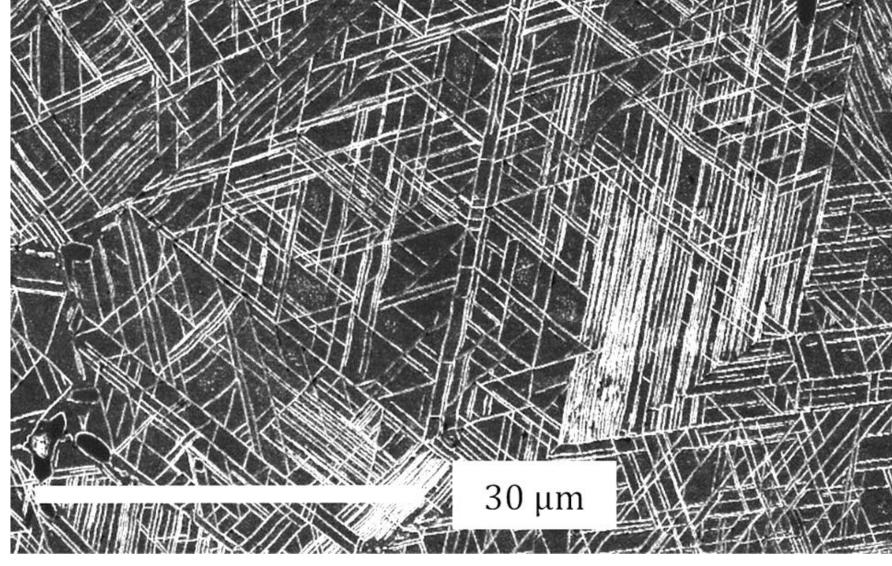
Fig. 2. SEM micrograph of an alloy based on Nimonic 263 containing only η phase in a Widmanstätten plate microstructure. Wong et al., 2015.
