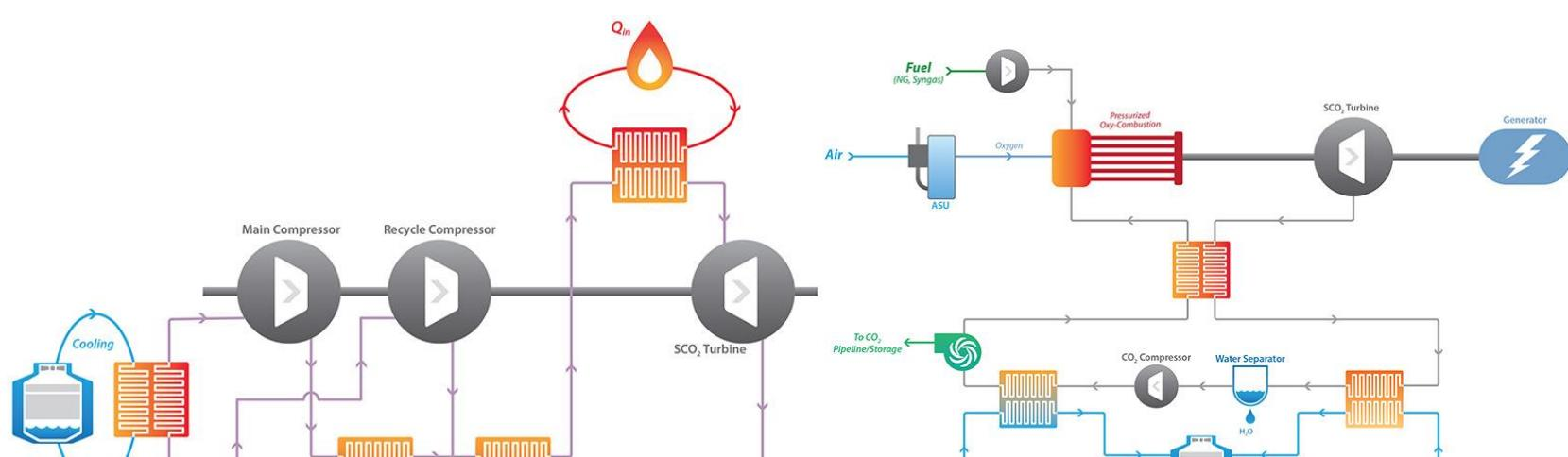
Indirect and directly fired supercritical CO<sub>2</sub> cycles
