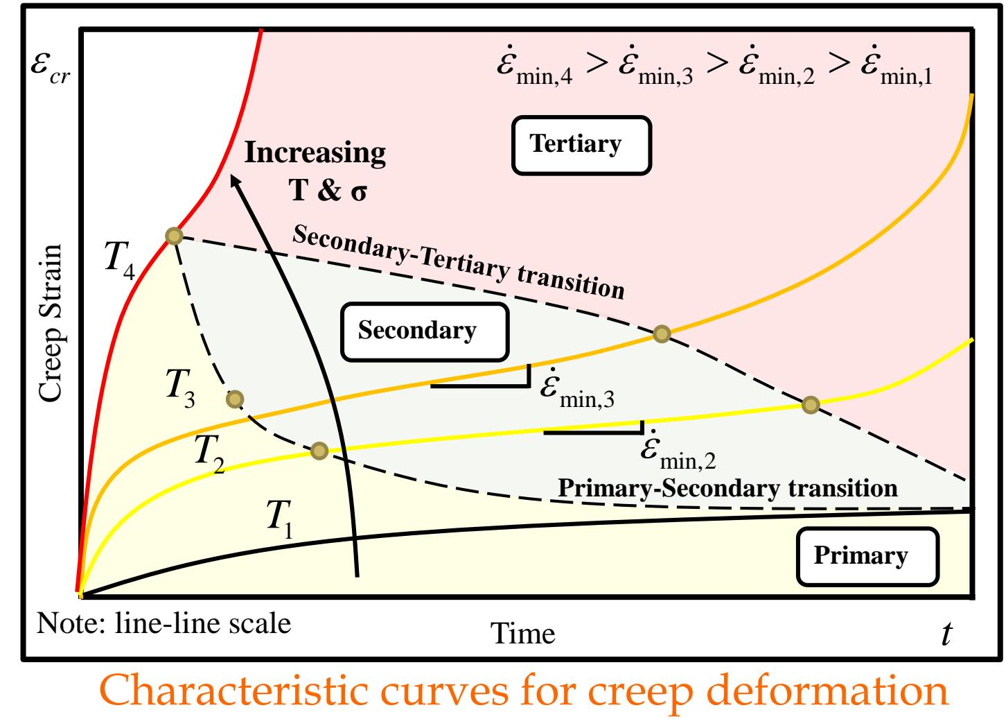
Characteristic curves for creep deformation
