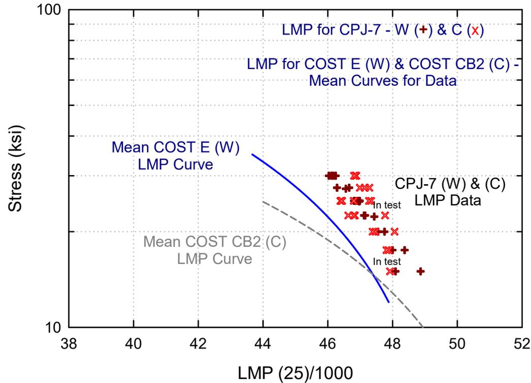
Larson-Miller Parameter plot for COST E & cast CB2 at temperatures from 1050°F (565.5°C) to 1200°F (648.9°C). CPJ-7 (cast (x) & wrought (+)) testing performed at 650°C only.
