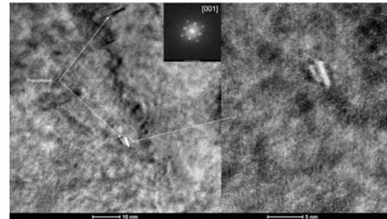
(Left) HRTEM micrograph showing fine coherent MX-type precipitates in the martensitic matrix of as-received CPJ 7. (Right) A magnified view of the lower precipitate in the left panel. The precipitate is located at the center of two high-strain (white) regions that result from lattice mismatch between the precipitate and the matrix.
