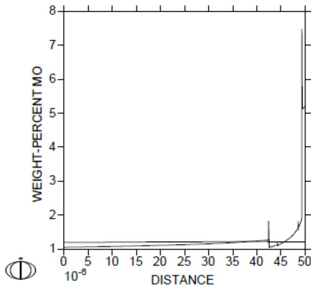
A plot of wt. % Mo vs. Distance (m) in the as-cast condition. It can be seen that there is quite significant difference in Mo weight fraction in the region equivalent to the center of, or  $\frac{1}{2}$ , the *sdas* length.
