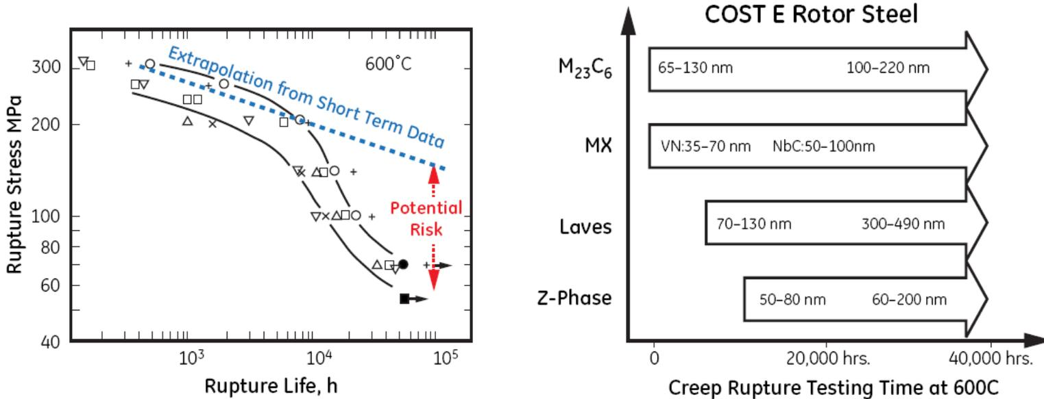
Many competing effects occur in heat resistant steels of the 9% Cr variety. Past experience has shown that the instability of any of the following, Z-phase, Laves, MX and/or M<sub>23</sub>C<sub>6</sub>, can cause an unexpected decrease in rupture stress as a function of time. The goal of alloy design is to slow down the destabilization of these features starting with the MX and M<sub>23</sub>C<sub>6</sub> particles.
