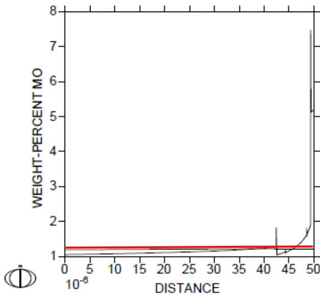
A plot of wt. % Mo vs. Distance ( $\mu\text{m}$ ) in the as-cast and homogenized condition. After homogenization the Mo level was  $\pm 1\%$  of the nominal level which was deemed adequate. Each element of the alloy was evaluated in a similar manner.
