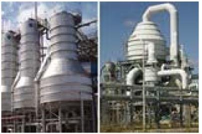
Mechanical Vapor Recompression and Crystallization
