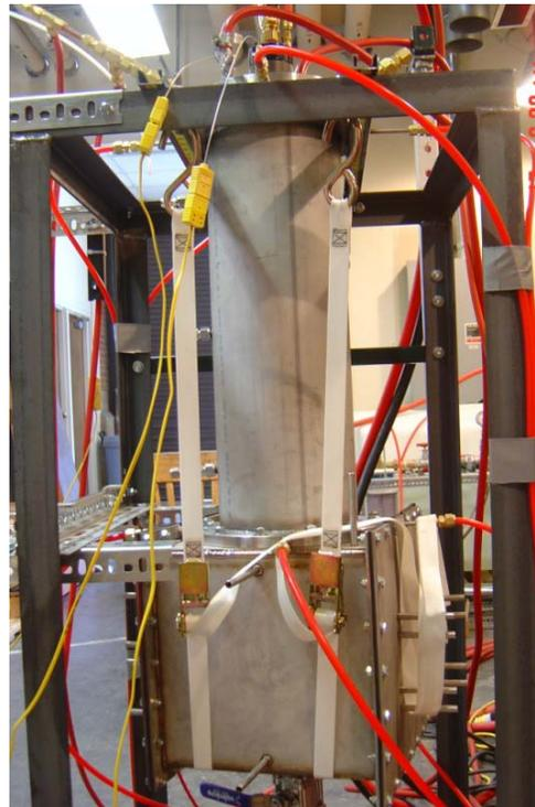
Water cooled reactor vessel
