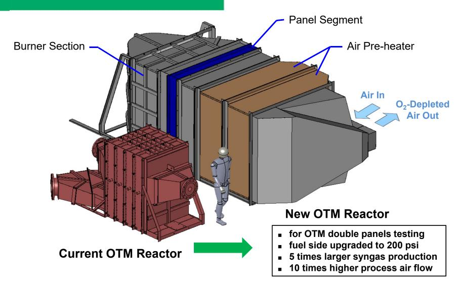
Larger Operation Capacity to Support OTM Double Panel Test
