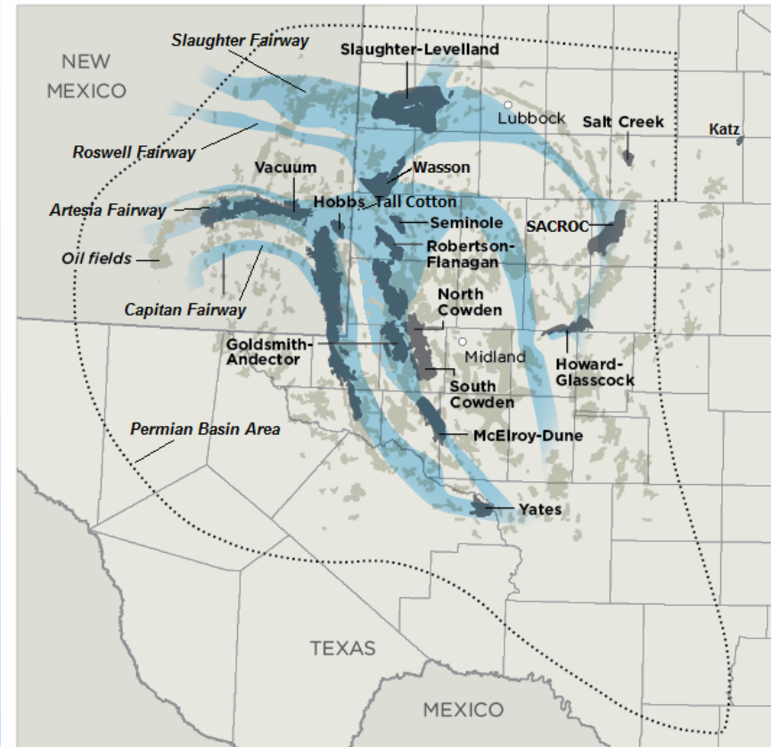
Residual Oil Zone Fairway Mapping with Superimposed Major Permian and Pennsylvanian Oilfields and Showing the First Pure ROZ Greenfield ROZ CO 2 Project
