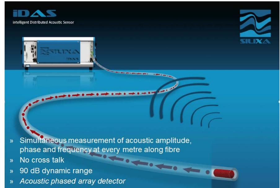
**A 10 km single mode fiber becomes a high density acoustic array with 10,000 linear sensors with 1 meter spatial resolution**
