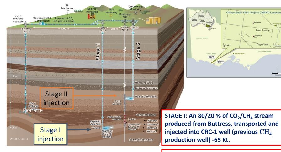
STAGE II: CO<sub>2</sub>/CH<sub>4</sub> stream injected into CRC-2 well – 15 Kt.
