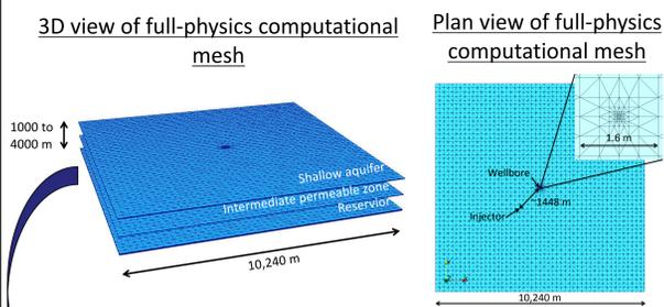
Example simulation of full-physics simulations of CO<sub>2</sub> leakage
