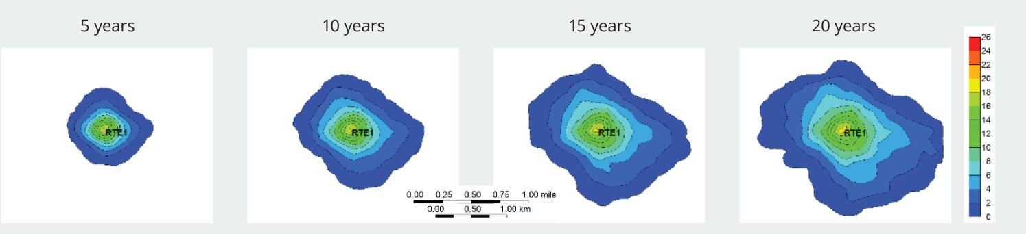
CO<sub>2</sub> plume evolution for the P50 (moderate) case after 5, 10, 15, and 20 years of CO<sub>2</sub> injection. Color changes in images represent changes in gas saturation. These reservoir simulation results were used to determine an anticipated area of review (AOR) for permitting and to constrain the horizontal and vertical requirements of a monitoring, verification, and accounting (MVA) program.
