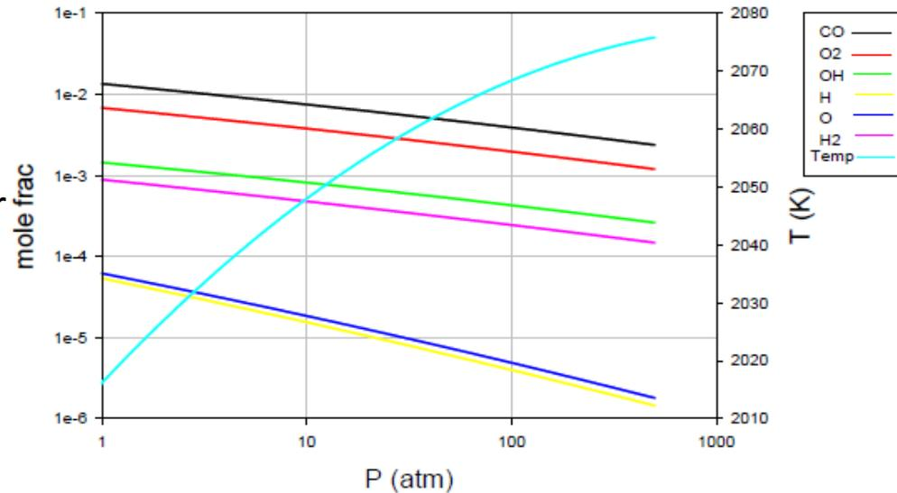
Effects of Increasing Pressure. Equilibrium calculation for CH<sub>4</sub>/O<sub>2</sub>/CO<sub>2</sub> at  $\phi = 1$ . Figure adapted from Strakey, 2014, sCO<sub>2</sub> symposium
