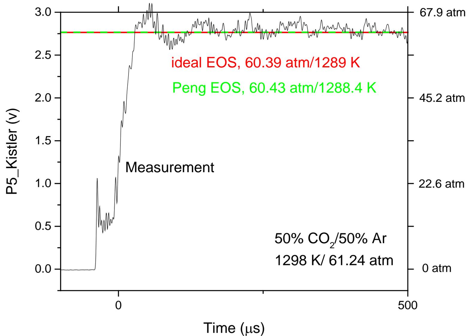
Reflected shock wave experiments: sidewall pressure profiles.
