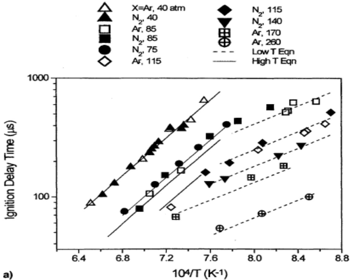
CH<sub>4</sub>/O<sub>2</sub>/N<sub>2</sub>/Ar ignition delay time measurements. The higher pressure data exhibit a significantly weaker variation with temperature (smaller activation energy) than the lower pressure, higher temperature mixtures
