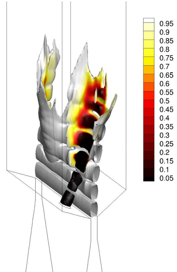
Iso-surfaces of  $M = 1.35$  shaded by equivalence ratio from 3D LES of single fuel-injector hole-pair.
