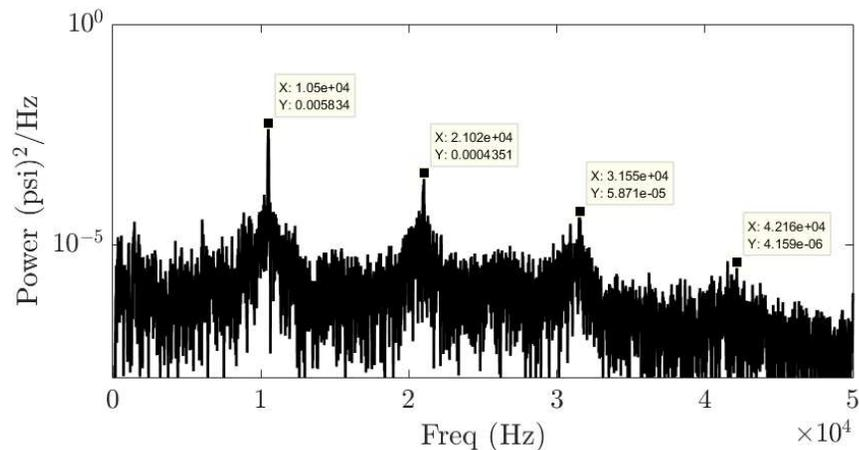
Combustion (T+50ms to T+100ms)
