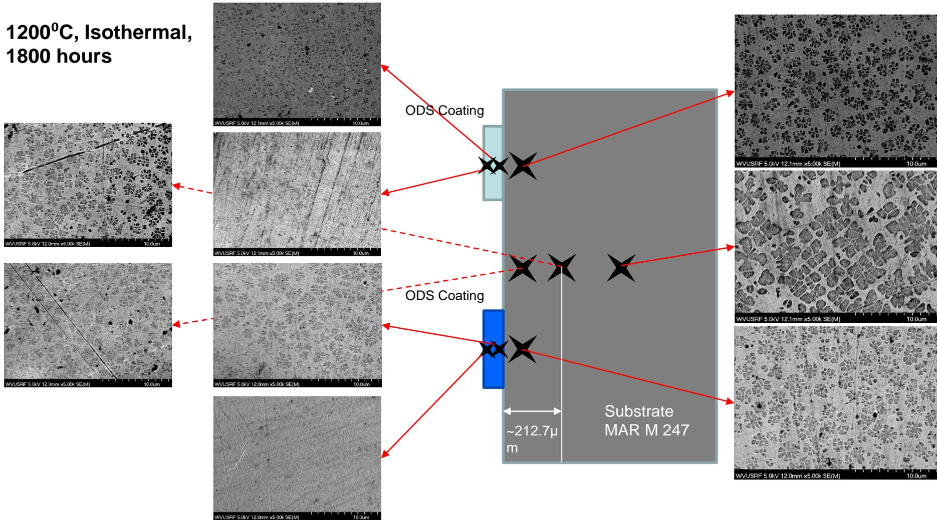
**\*\*Gamma Prime ( $\gamma'$ ):** This phase constitutes the precipitate used to strengthen the alloy. It is an intermetallic phase based on  $Ni_3(Ti,Al)$  which have an ordered FCC L12 structure
