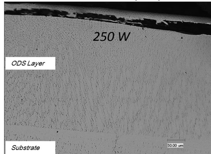
*Cross Section of Laser Deposited Samples*
