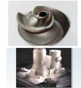
*As metallic additive manufacturing technologies advance significantly over the recent past, complex metal products, such as turbine components, can be manufactured by this innovative technology.*
