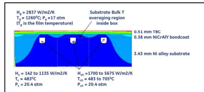
Skin Cooled Bulk Substrate Metal Temperature as a Function of Channel Heat transfer Coefficient and Coolant Temperature
