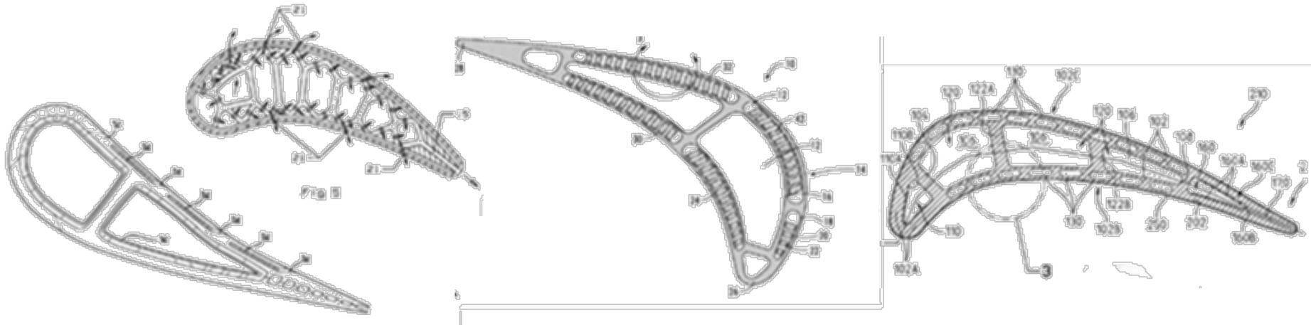
Different patents showing double wall cooling by UTC, Siemens and Florida Turbine Technologies
