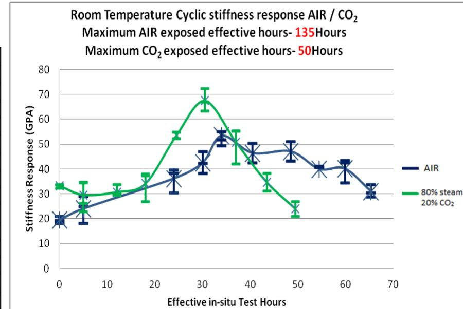
In-situ micro-indentation stiffness response of APS/MCrAlY/RenéN5 coupon under cyclic oxidation room to 1100°C under **air** and **wet (80% steam/20% CO<sub>2</sub>)** conditions
