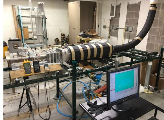
Test Rig for Conjugate Heat Transfer
