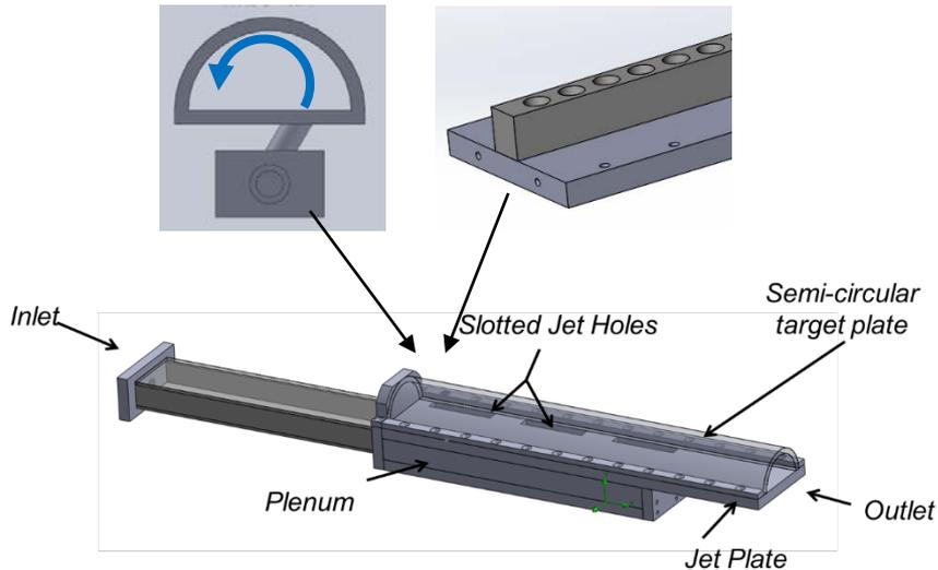
“Screw” Cooling Concept for Leading Edges
