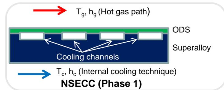
ODS Coupons with Rectangular Cooling Channels
