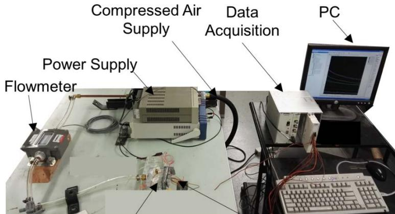
Test Section Thermocouples
