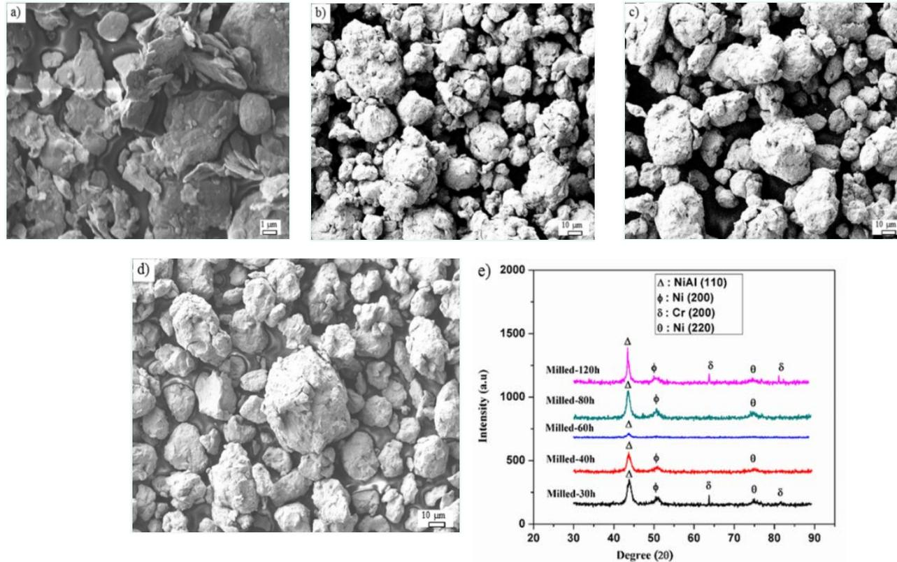
SEM micrographs of milled ODS powders for (a) 5 hrs, (b) 40 hrs, (c) 60 hrs, (d) 120 hrs, and (e) XRD spectrum.
