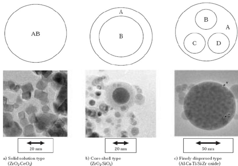
**Structural patterns of nanocomposite particles**
